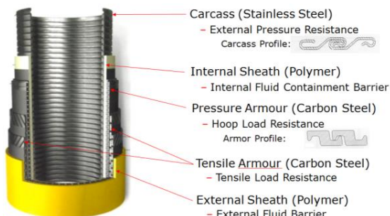
Figure 1. Cross-section of a flexible marine riser.
